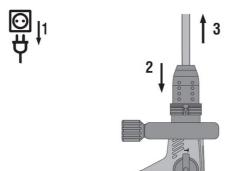
Pull the chuck back as far as it will go and remove the accessory tool.
