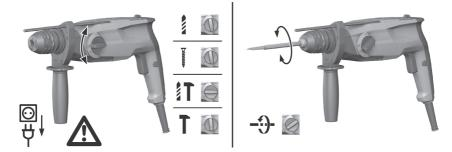
► Set the function selector switch to the "Drilling with hammering action" (hammer drilling) position (T.
