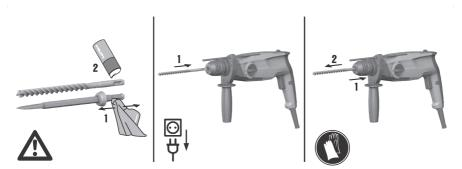
Fit the drill bit or other accessory in the quick-release chuck or, respectively, remove the drill bit or other accessory from the quick-release chuck.
