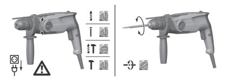
► Set the function selector switch to the "Chisel positioning" position -Э.
