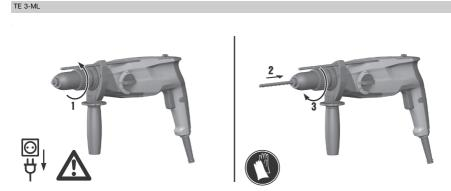
► Fit the drill bit or other accessory in the three-jaw chuck or, respectively, remove it.
