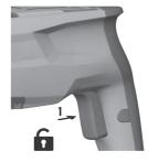
Press and lock the control switch.
