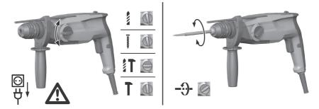
► Set the function selector switch to the "Drilling without hammering action" position 2.
