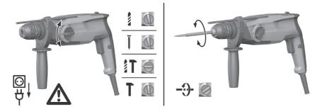
• Set the function selector switch to the "Chiseling" position  $\mathbf{T}$ .
