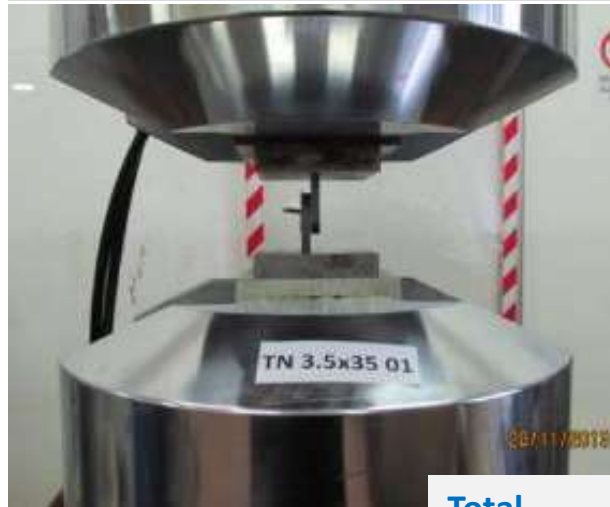
Shear tests on self-tapping and self-drilling screws
