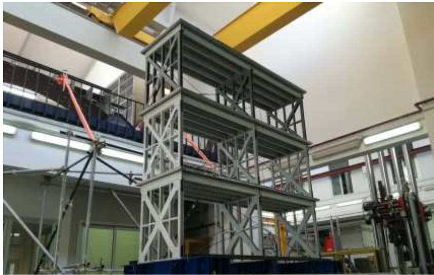
Prototype with composite steel-concrete floors
