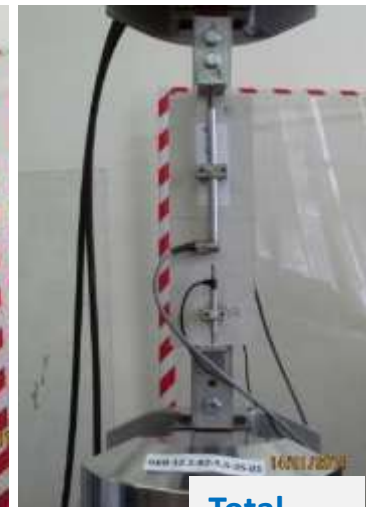
Shear tests on screwed panel-to- steel connections
