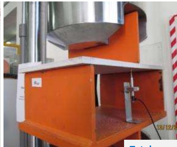
Bending tests on sheathing panels
