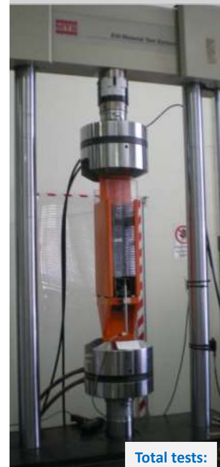
Tests on hold-down devices
