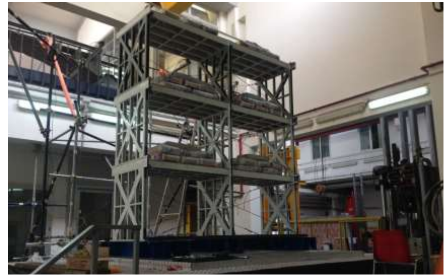
Prototype with wood-based (OSB panels) sheathing braced floors
