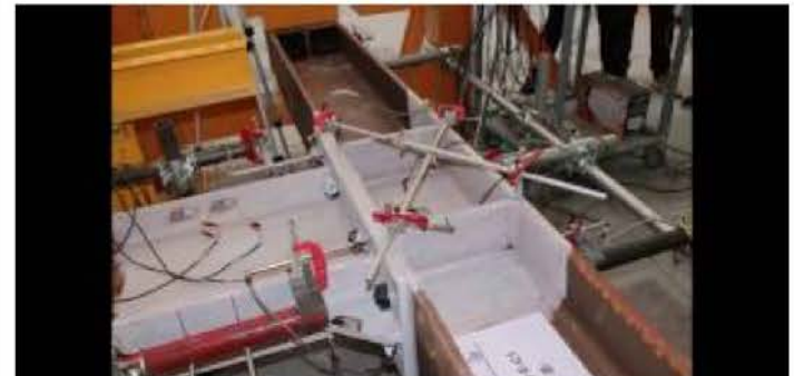
Stiffened extended endplate beam-to-column joint ES2-TS-E-C1 2018-11-09
