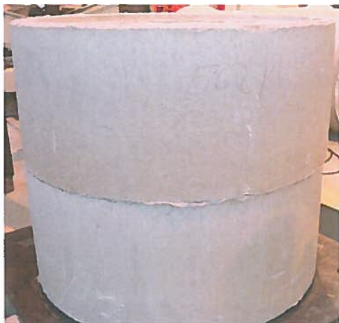
Pictures 3 and 4: View of the manhole rings after assembly with foam outlet on the outside and inside
