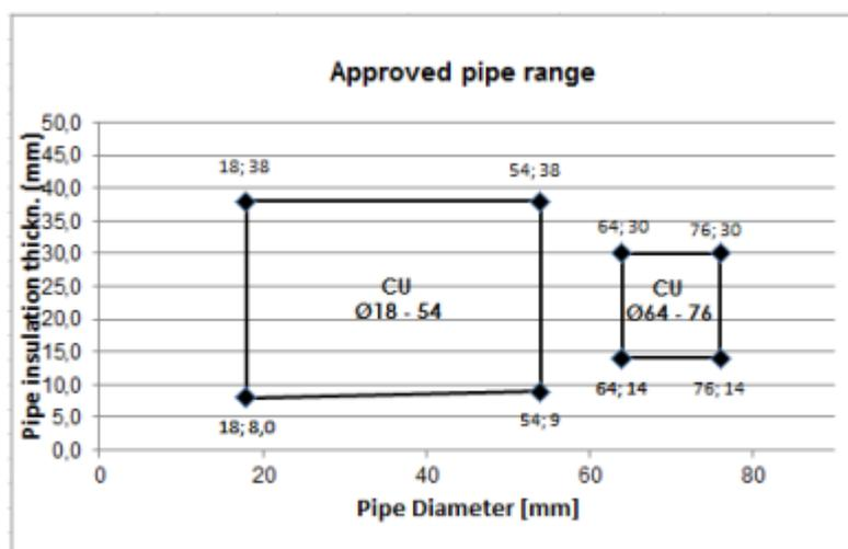
**2.2.11 Copper pipes including metal pipes,
